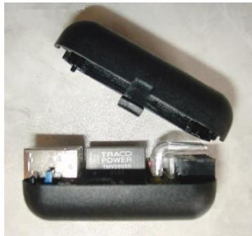
*Start fastening the top cover on the edge closer to the LEDs. Then fit the top cover onto the bottom cover with slight power.*
