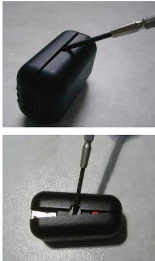
*Carefully lever up the device at both grooves using a small screw driver. Remove the top cover carefully.*
